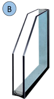
Double glass windows U_g = 3.2 \text{ W/m}^2\text{K}
