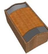
Displacement incompatibility between diaphragm and URM end walls.
