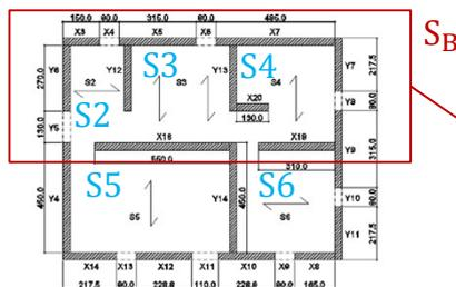
$$F_{AS_2} = F_{A,SB} \cdot \frac{G_{d,0}^{S_2} \cdot B_{S_2}}{G_{d,0}^{S_B} \cdot B_{S_B}} = 57.67 \cdot \frac{150 \cdot 2.35}{346 \cdot 10.80} = 5.45 \text{ kN}$$
